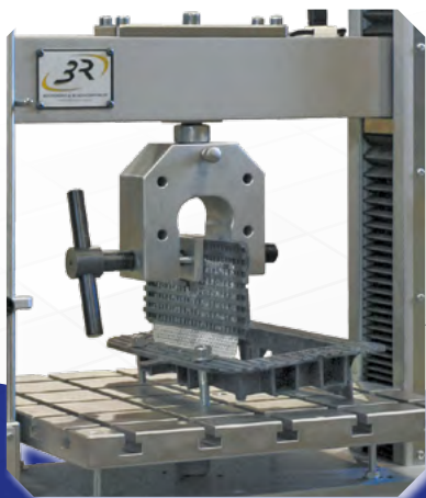
An airbag hatch resistance test
