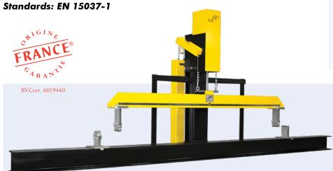
Aimed for pre-stressed or reinforced concrete beam producing factories, our machine allows one operator to run the different tests in an **automatic modus**, including the load stages prescribed by the EN 15037-1.
